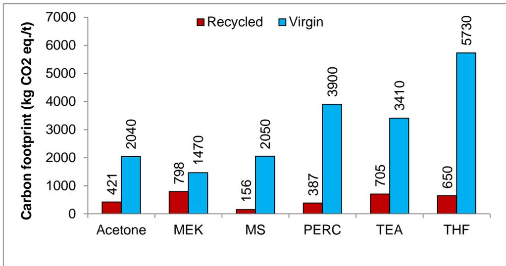
**Figure 3 Carbon footprint of recycled and virgin solvents [3]**
